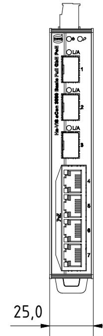
for mounting rail acc.to DIN EN 60715
