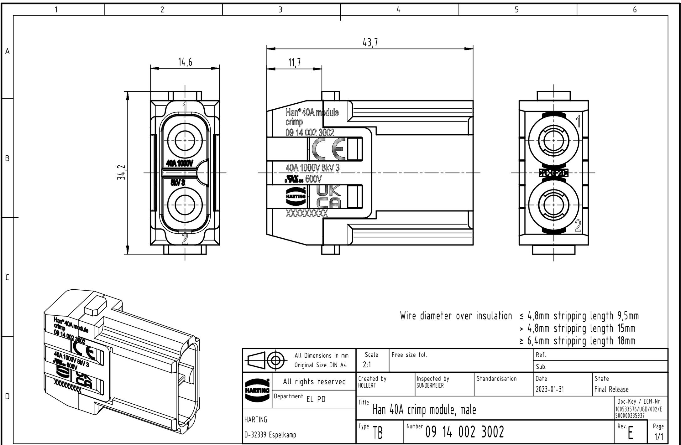
Wire diameter over insulation  $\leq 4,8\text{mm}$  stripping length 9,5mm
